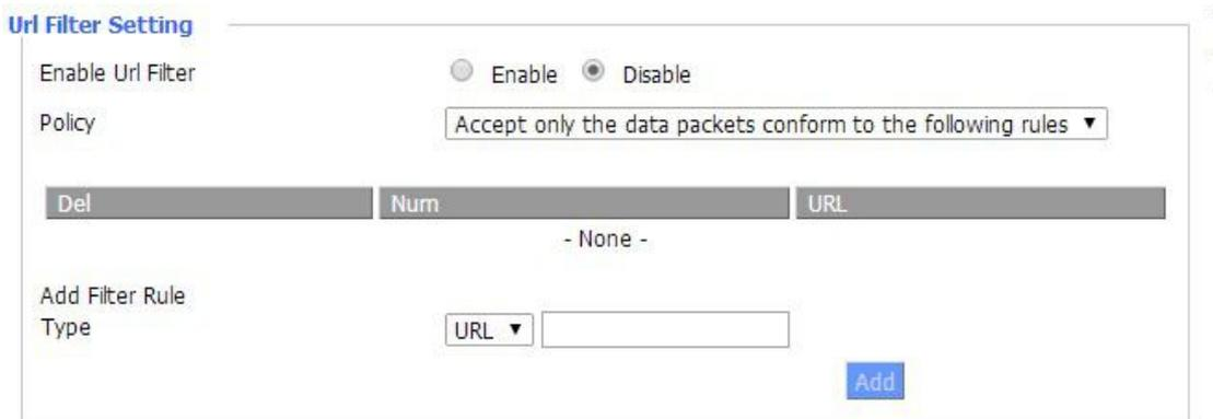
The screenshot shows the 'Url Filter Setting' configuration page. At the top, there are radio buttons for 'Enable' and 'Disable'. Below that is a 'Policy' dropdown menu. A table with three columns: 'Del', 'Num', and 'URL' is shown, with '- None -' in the 'Num' column. At the bottom, there is an 'Add Filter Rule' section with a 'Type' dropdown menu and an 'Add' button.
