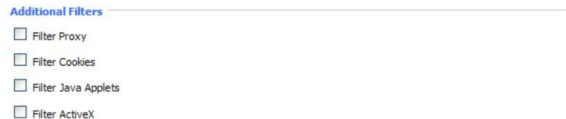
**Filter Proxy:** Wan proxy server may reduce the security of the gateway, Filtering Proxy will refuse any access to any wan proxy server. Click the check box to enable the function otherwise disabled.
