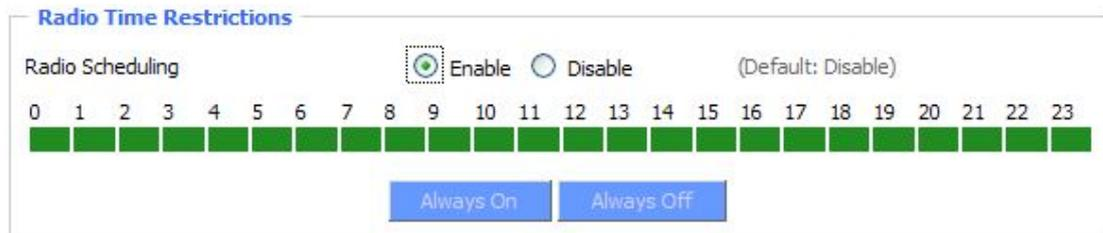
**Radio Time Restrictions:** The *Radio Times Restriction* facility constitutes a time switch for the radio. By default, the time switch is not active and the WLAN is permanently on. Enable the time switch, if you want to turn off the WLAN during some hours of the day. Hours during which the WLAN is on are marked in green, while red indicates that the radio is off. Clicking on the respective hour toggles between on and off.
