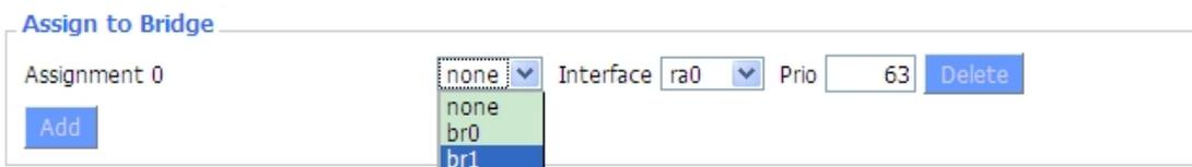
Assign to Bridge option: to assign different ports to created bridge. For example: assign port (wireless port) is ra0 in br1 bridge as below:
