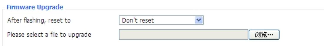
**Firmware Upgrade:** New firmware versions are posted at [www.four-faith.com](http://www.four-faith.com) and can be downloaded. If the Router is not experiencing difficulties, then there is no need to download a more recent firmware version, unless that version has a new feature that you want to use.
