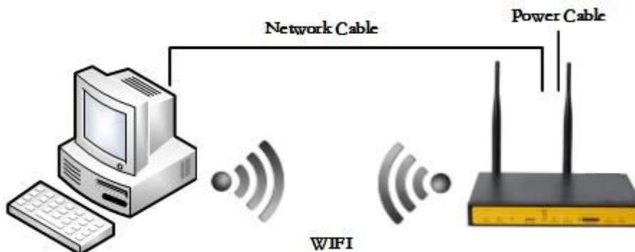
Please modify the IP address of PC as the same network segment address of the router, for instance, 192.168.1.9. Modify the mask code of PC as 255.255.255.0 and set the default gateway of PC as the router's IP address (192.168.1.1).
