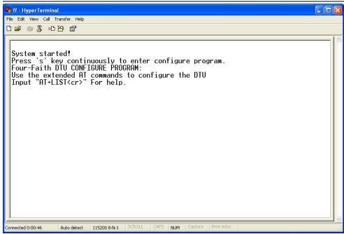
7. IP MODEM has entered configure state, you can configure the parameters through AT command.
