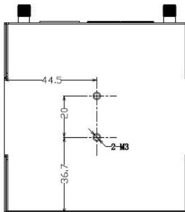
DIN Rail installing position
