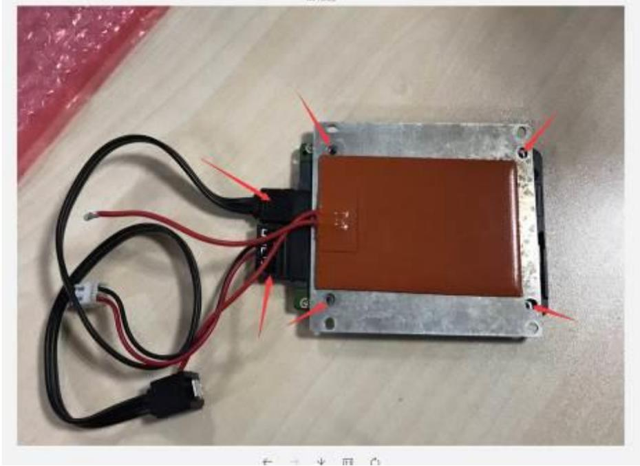
3. Fix the hard disk on the device and connect the power supply and data cable.
