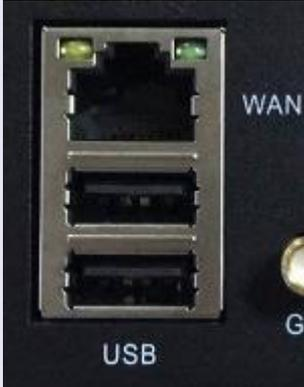
A panel with a WLAN port (RJ45) at the top, two USB2.0 ports in the middle, and a small circular port labeled "G" at the bottom right. The label "USB" is at the bottom. | WLAN<br>USB                                                 | RJ45<br>10M/100M/1000M adaptive Ethernet port.<br>USB2.0: supports mouse and USB flash drive access. |
