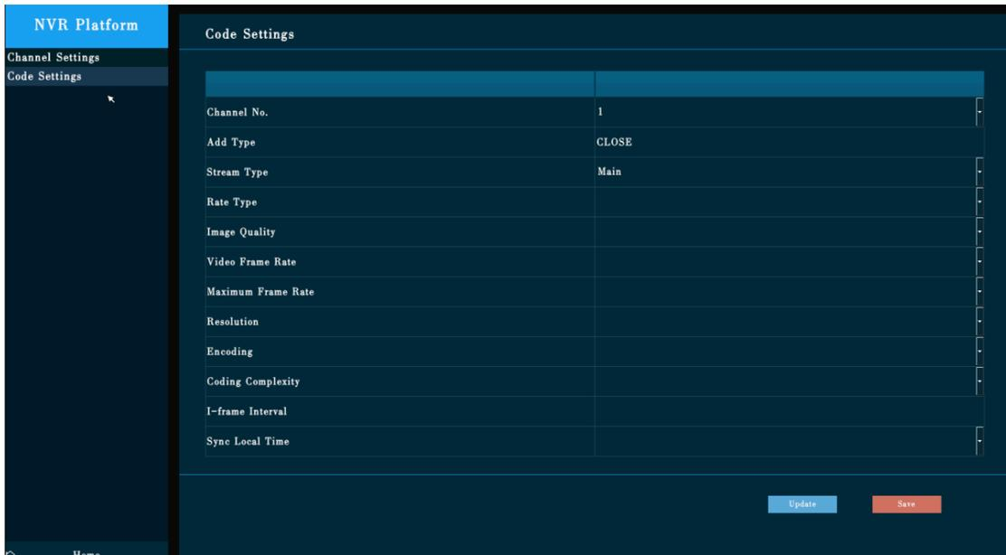
On the code settings interface, user can edit the parameter such as stream type, rate type, video frame rate, maximum frame rate and so on
