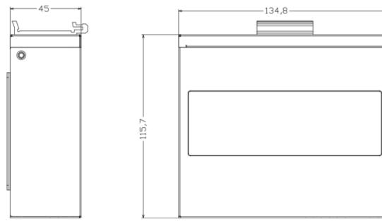
Note: The screw of the switch installed with the fixing plate is M3, and the depth of the screw locking into the switch is 3-4mm.
