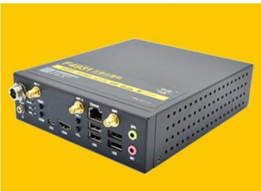
F4931-R2H is a low-power industrial computer independently developed by Four-Faith. It combines wireless cellular network and routing technology with industrial computer technology.
