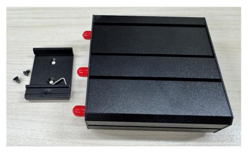
**Step 1:** Flip the IWR202 to its back side and take out the DIN rail bracket and two screws from the rail tool kit.
