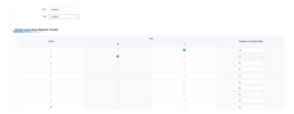
The VLAN feature enables users to segment ports based on their preferences. The system supports up to 15 VLAN ports (VLAN1 to VLAN15), but only two ports can be configured: one for WAN and one for LAN. These ports can be assigned to different VLANs as needed, but the LAN and WAN ports cannot belong to the same VLAN.
