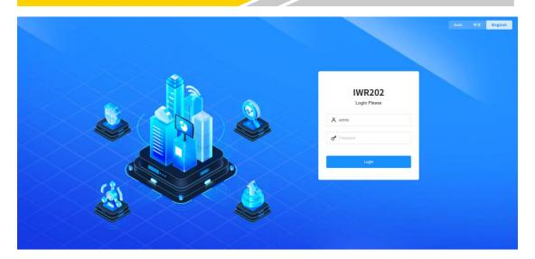
To access the router's web-based management interface, launch Internet Explorer or any other web browser. Refer to Section 2.2.1 for the appropriate access method, then enter the corresponding URL in the address bar. Use the default username and password, both set to admin, to log in and configure the router's settings.
