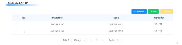
Allows you to add and manage multiple LAN IP addresses and subnet masks, enabling devices within corresponding IP segments to connect to the network.
