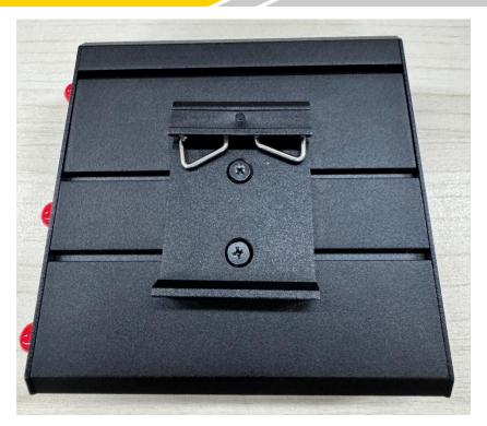
**Step 3:** Secure the bracket with the supplied screws and tighten them to complete the installation.
