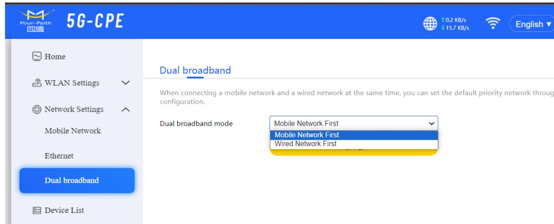
Insert the SIM card into the device and connect the LAN2/WAN port to the upstream device as the WAN port. The device will prioritize using the mobile network. When the mobile network is unavailable, it will automatically switch to using the Ethernet connection.
