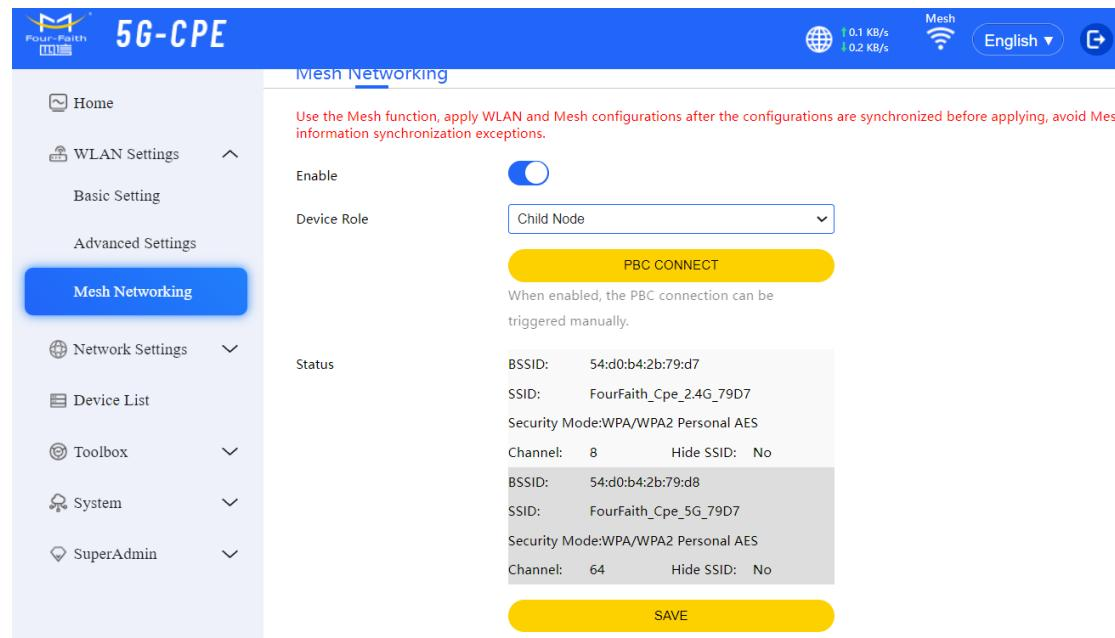
The screenshot shows the 'Mesh Networking' configuration page. The left sidebar has a 'Mesh Networking' button highlighted in blue. The main area shows the following settings:
