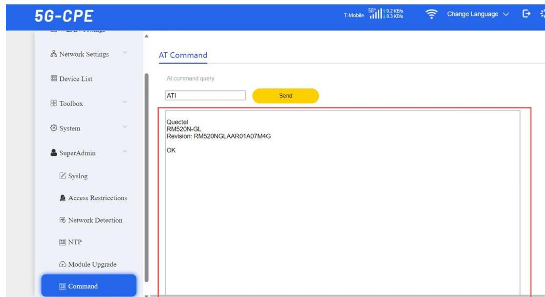
This screenshot is identical to the one above, showing the 5G-CPE configuration interface. The 'Command' button in the sidebar and the response area in the main panel are highlighted with red boxes. The response area displays the device's details and the status 'OK'.
